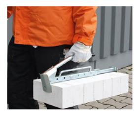
Rugged tubular steel construction for the transportation of engineering bricks from the pallet to the place of use by hand.
